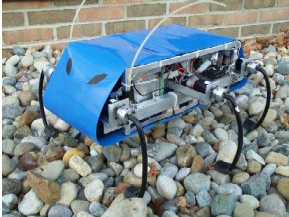
Figure 22: RHex walks through gravel 24
