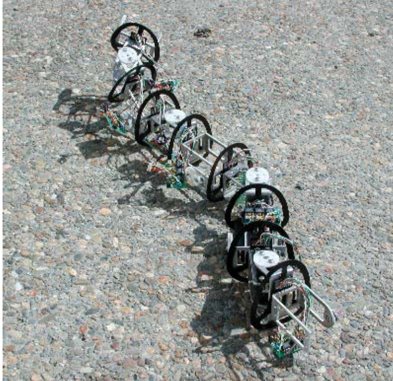
Figure 23:A Third-Generation Model of a Snake-bot Being Developed for Mars Exploration 26
