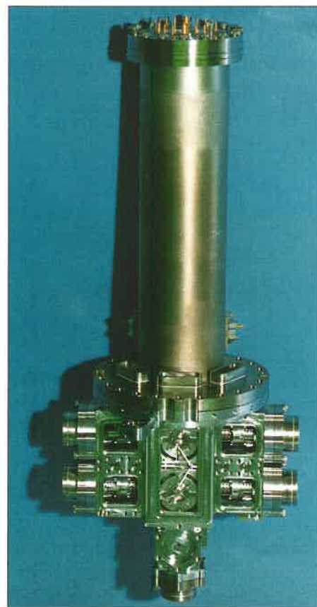
Fig. 7. The ion source system, showing the individual ion sources and the switching lenses in the partially assembled ion source housing before installation of the getter housings and the gas inlet manifolds. The overall length is 357 mm.
