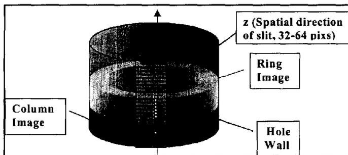
Fig. 1. Sketched description of the column and ring mode of MA\_MISS
