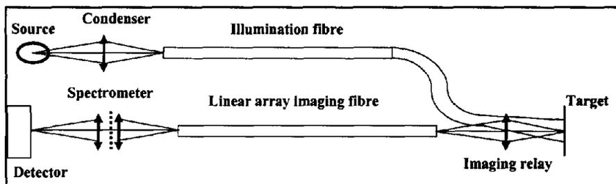
Fig. 2. Simultaneous spectral detection spectrometer concept.
