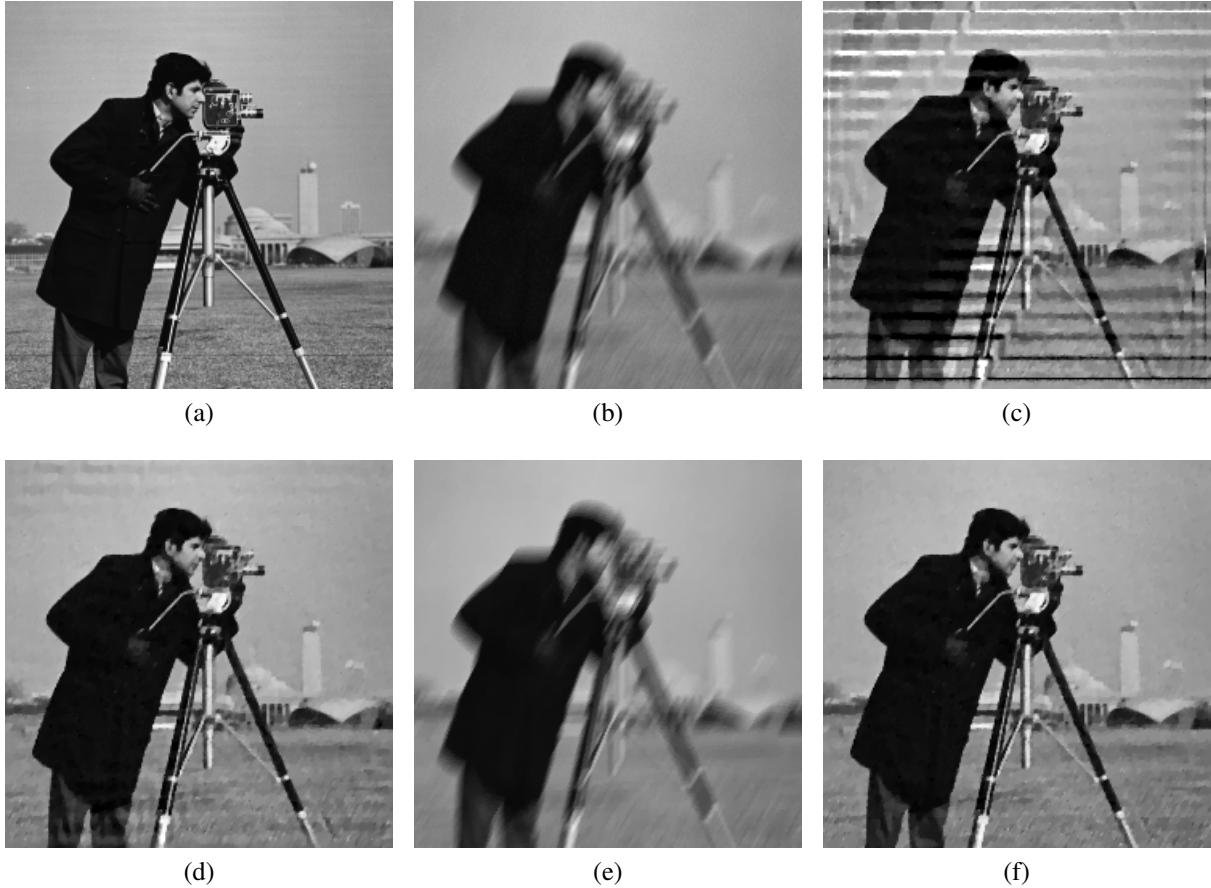
Figure B.2: Experiment 3 using 15 pixel motion blur: Restoration results using isotropic TV regularization. (a) Cameraman true image ( 248 \times 248 ), scaled to the range [0, 1] . (b) Blurred and noisy image from Matlab's 'valid' conv2 operation. (c) Restored image from purely circulant model (B.2). (d) Restored image from purely circulant model with data pre-processing (B.4). (e) Restored image using reflexive boundary conditions and DCT (B.5). For this case, the results are inaccurate since this method is not applicable for non-symmetric PSF [4, 5]. Also the image had to be scaled to fit the dynamic range of the rest of the reconstructed images. (f) Restored image from proposed non-circulant model (B.8).
