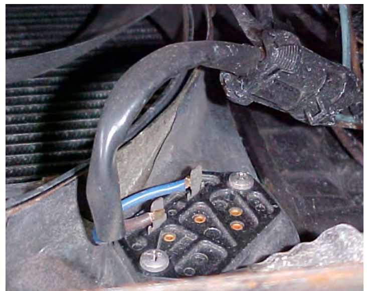
This is what the resistor looks like (with winter salt)
