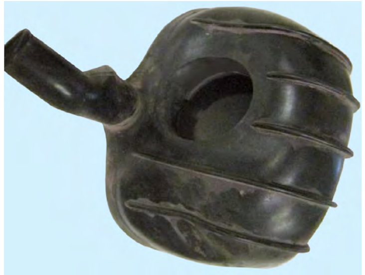
Rubber boot; the fuel filler goes through the big hole. The tube goes through the trunk floor to drain refueling spills.
