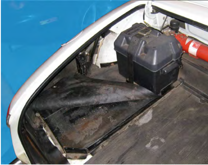
Spider fuel tank area. Note battery mounted to reinforcement.
