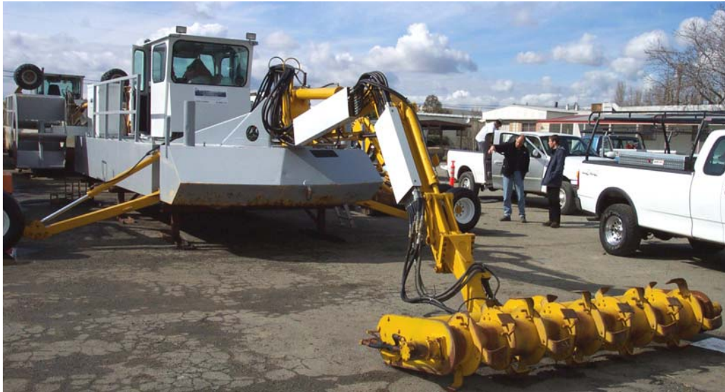
Aquamog: underwater rototiller (Aquatic Environment)
