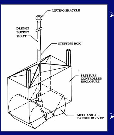
Pressure-controlled housing provides a dry environment around the mechanical bucket or mixing in-situ treatment zone
