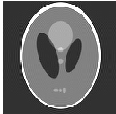
(a) Fourier reconstruction from Cartesian samples
