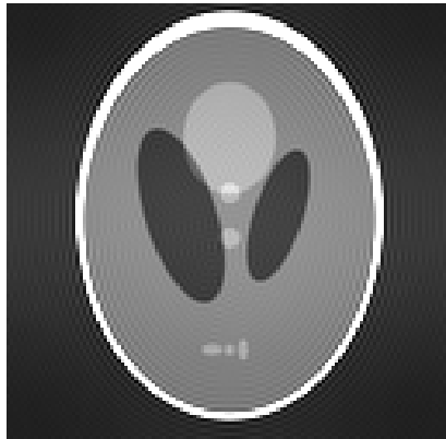
(a) Fourier reconstruction from Cartesian samples
