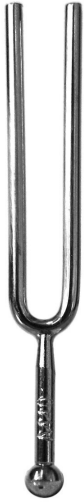
Figure 2.14: A tuning fork that, when struck, reliably produces a note with frequency 440 Hz.
