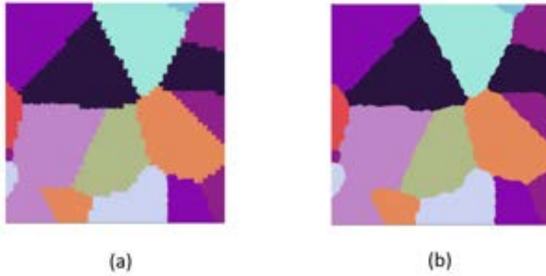
Figure 2.4: Grain identification in a mesh using a 50x50 pixel image: (a) Pixel-based labeling (b) Multiway K-Cut based labeling.
