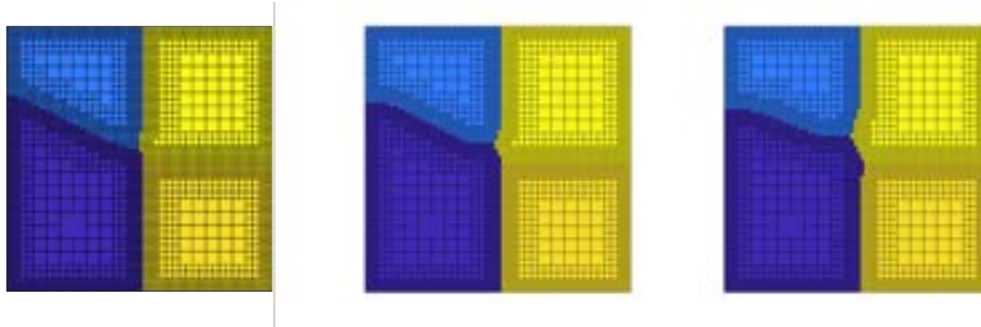
Figure 4.6: A 4-point junction splitting into 2 3-point junctions. All grains have no bulk energy density and surface energy between each pair of grain is also same.
