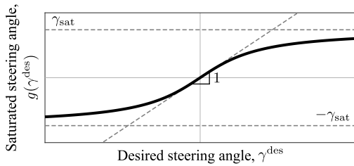
Fig. 6. The continuous wrapper function g(\gamma^{\text{des}}) in (18).
