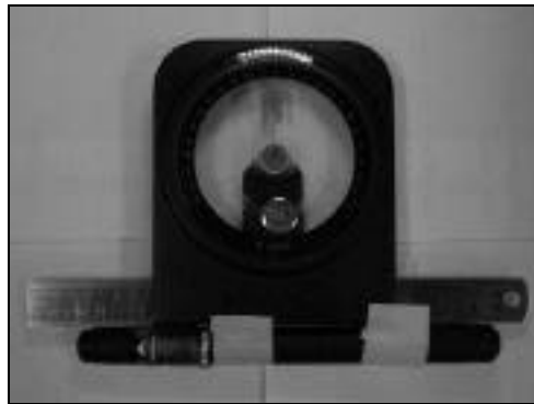
Figure 30. Inclinometer with a laser pointer attached
