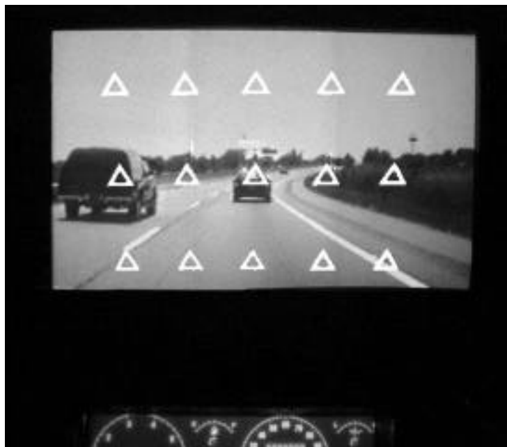
Figure 2. All 15 locations of the HUD activated with the road scene. The color of the triangles was changed to white in this figure for clarity.
