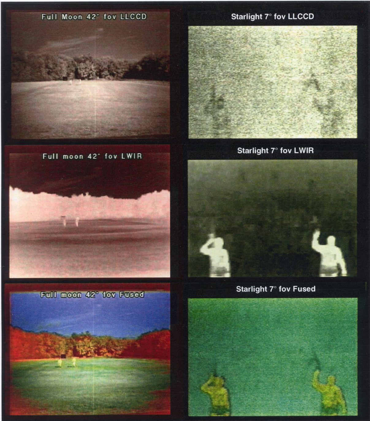
Color night vision by realtime fusion of low-light CCD visible and uncooled LWIR thermal imagery. Taken under full-moon (100mLux) conditions near Lincoln Laboratory using 42° field-of-view optics. Men are located at about 100m, background trees at over 200m from the sensor pod. (Top) low-light visible, (middle) LWIR, (bottom) fused imagery.
