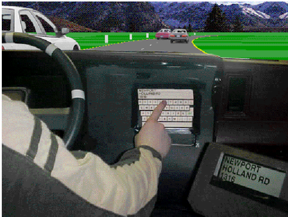
Figure 6. Driver's view of the road and touch screen (Note: The touch-screen keyboard and road scene were enhanced in this image for clarity)
