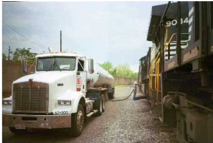
Figure 3: A fueling truck refueling a locomotive.
