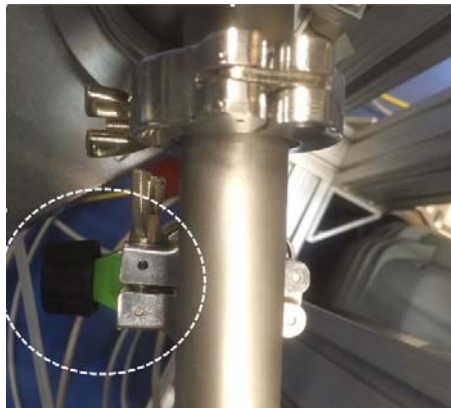
Figure 5: A picture of the vent valve, MV-3, of vacuum pump system under the chamber.
