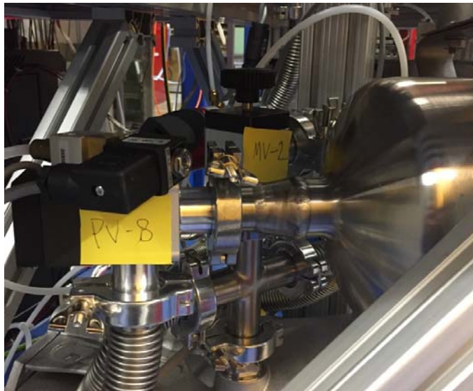
Figure 10: A picture of MV-2 between PV-5 (not pictured) and the target cell.
