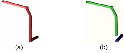
Figure 5. (a) infeasible component with an out-of-plane bend and (b) feasible components without out-of-plane bends.
