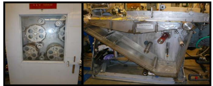
Figure 4. PAPER TOWEL PILOT MACHINES: TOWEL FORMER ON RIGHT, TOWEL DRYER ON LEFT
