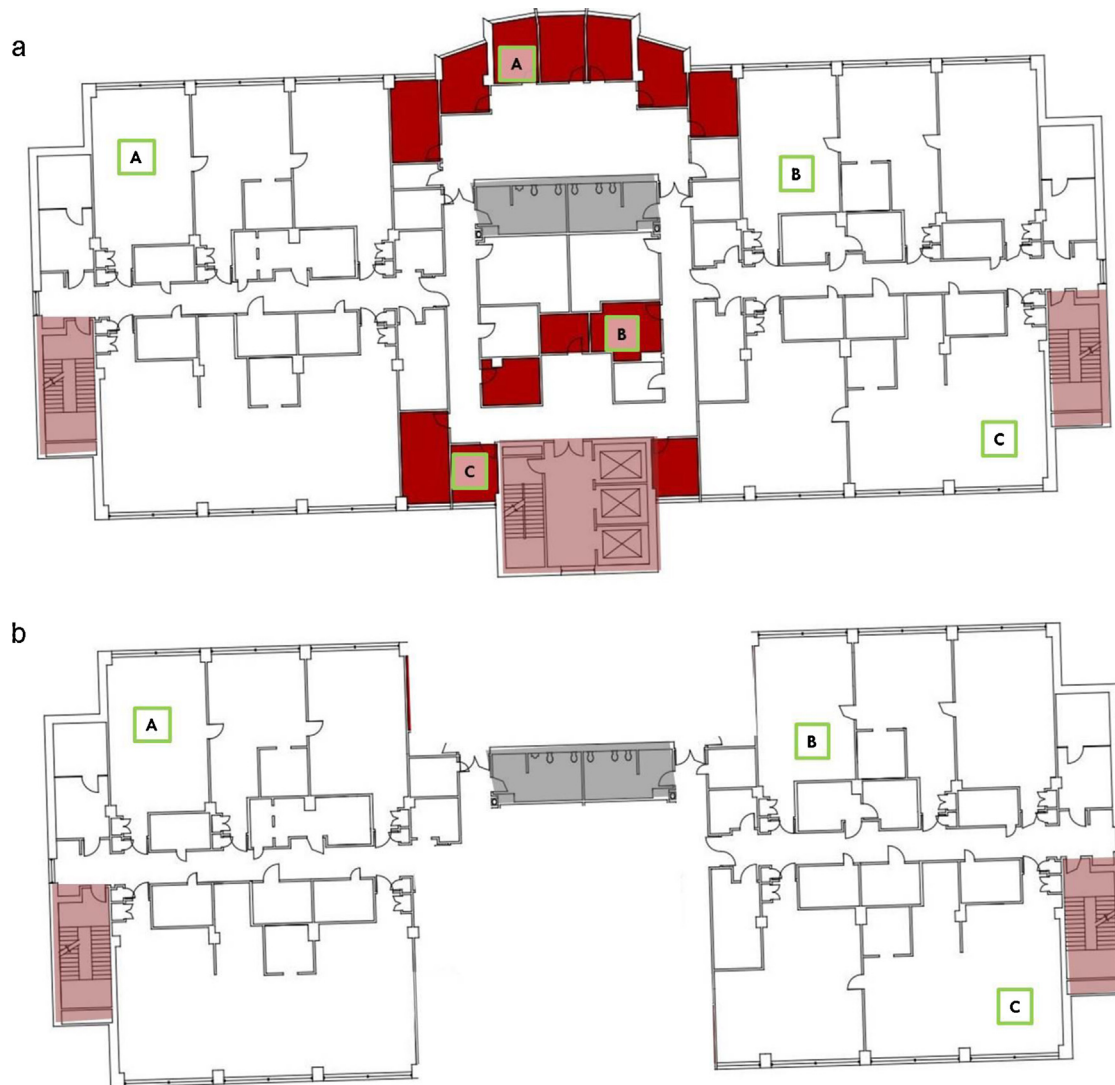
Fig. 4. (a) Offices (in red) in BLD2 are clustered around the core of the building. The connections between offices and other spaces are on the basis of immediate adjacency, which is a more direction connection than in BLD1. (b) The effect of removing offices in BLD2 is to nearly sever the two wings or ends of the floor plan. This has a significant impact on the overlaps between researchers, and is likely to be even more pronounced in instances where ingress and egress onto the floor is through the two staircases on either end of the floor. (For interpretation of the references to color in this figure legend, the reader is referred to the web version of the article.)
