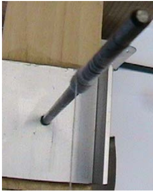
Left: Top (friction) bearing.
