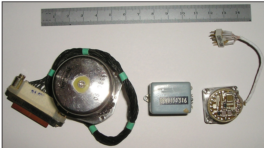
Figure 28. MG-4 gyroscope, AK-5 and A-15 accelerometers.
