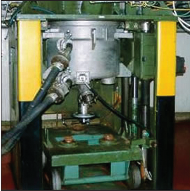
Figure 8. 30-gallon/100-liter propellant mixer bowl.
