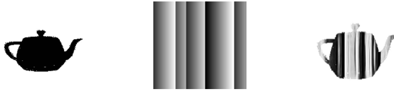
Figure 11. Painting texture onto a teapot. Left: Binary Mask of teapot; Middle: Texture; Right: Painted teapot
