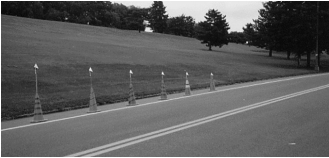
Fig. 2. Roadside-deployed basic {111111} array of radar-reflecting corner cubes
