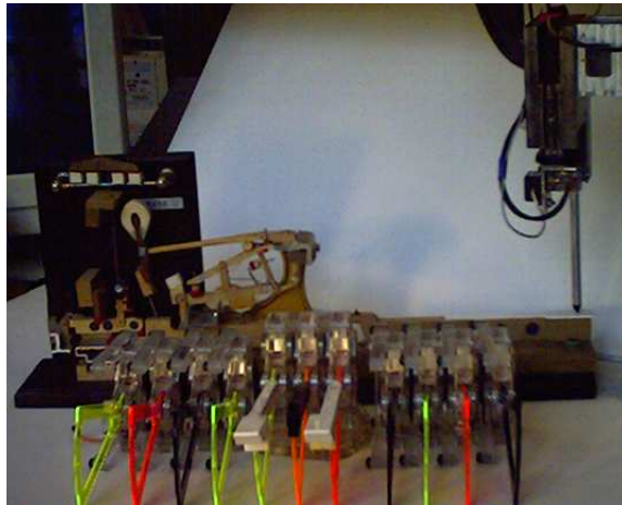
Figure 1. On the right a motorized instrumented probe presses on a piano key. In the foreground a prototype force reflecting synthesizer keyboard is visible.
