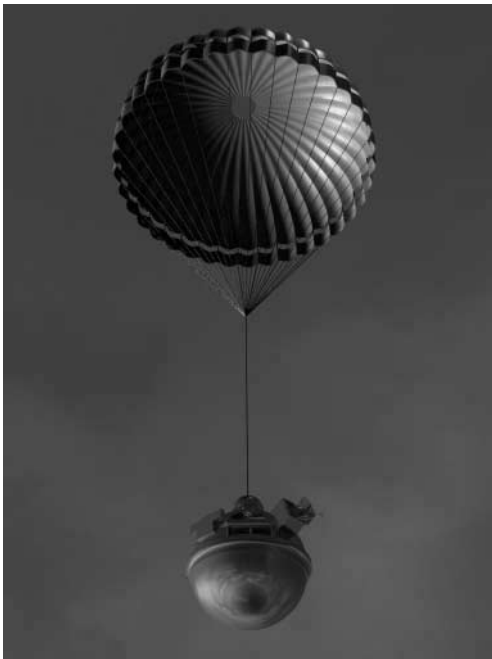
Fig. 7 Probe missions to Venus and the giant planets would descend under a parachute while performing descent science measurements (Credit: T. Balint)
