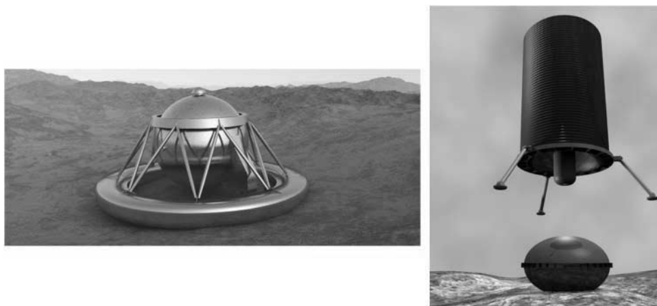
Fig. 10 Left: Venus lander concept from the Venus flagship mission study. The lander would use a rotating pressure vessel with a permanently mounted sample acquisition system and panoramic camera. Right: Venus mobile explorer concept, showing the inflated metallic bellows ascending to a float altitude of \sim 5 km, leaving the empty helium tank at the landing site (Credit: T. Balint)
