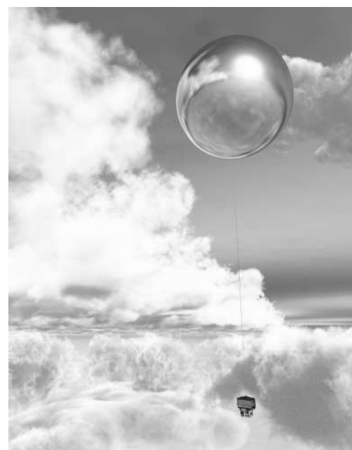
Fig. 9 Artist's concept of a superpressure Venus balloon, performing 30-day science investigations while circumnavigating the planet several times at a float altitude of \sim 55 km (Credit: T. Balint)
