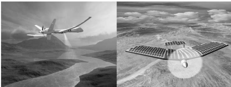
Fig. 13 Airplane concepts for Titan (left, AVIATR, reference [32]) and Venus (right, reference [33]). Both concepts can be used in the highly dense atmospheres of Titan and Venus.
