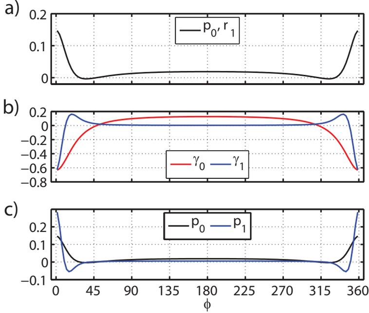
Fig. 4. A comparison of zeroth and first order terms in the solution for the point vortex located at  $a = 1.5$ , translating near a flexible circular wall which deforms according to linear elasticity:  $k(r(\phi) - 1) = [p](\phi)$ . The first order radial position is thus the same as the zeroth order pressure.
