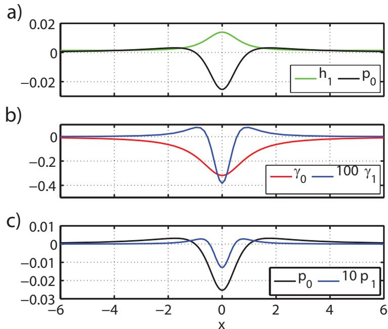
Fig. 2. A comparison of zeroth and first order terms in the solution for the point vortex translating near an infinite flexible wall which is a constant tension membrane over a deformable substrate:  $k(-\partial_{xx}h + h) = -[p]$ .
