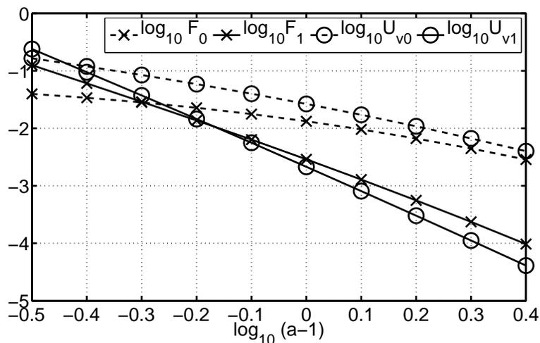
Fig. 5. For a point vortex moving near a deformable circular wall, and as functions of the vortex radial position  $a$ , the zeroth and first order terms in the total force on the circular wall  $F = F_0 + \frac{1}{k}F_1 + \dots$  and the vortex speed  $U_v = U_{v0} + \frac{1}{k}U_{v1} + \dots$
